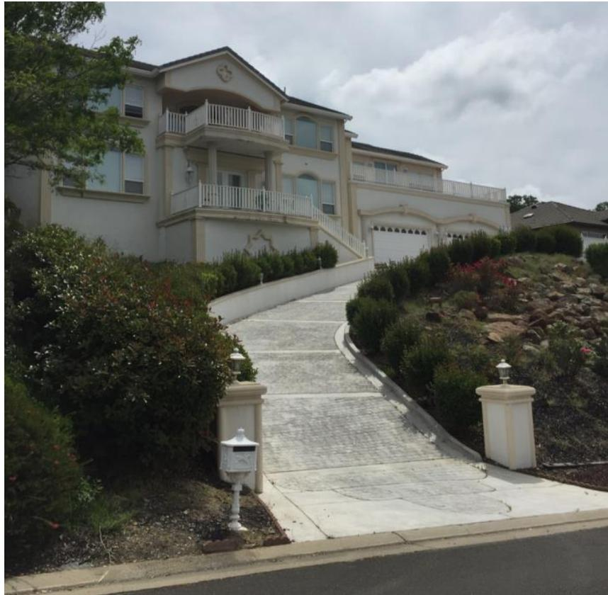
In a typical ascending home, the top of the house is about five stories from the street level requiring the aerial ladder for access. In some cases, it is faster to use the ladder for front-door access and water supply.
